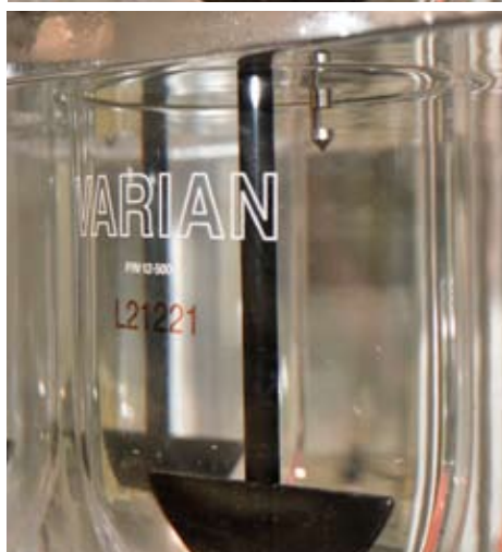
Fiber-optic probe in sampling and raised positions (top and bottom, respectively) to minimize hydrodynamics during the test.
